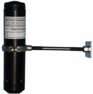
When mounting the Sonic Wave Sensor XB, a level should be used to assure it is vertical. The unit should be mounted such that the ultrasonic air space is at least 0.25 meters away from any objects. However a flat vertical surface may be closer in some cases. The unit should stay at least 0.2 meters above the water.
