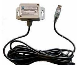
XB to USB Adapter Waterproof (IP67) with 5 meter long cable. Part #OSSI-015-020/020 Pro for North America with a RF Line of Sight Range of 2 miles and Indoor/Urban Range of 300 ft. and OSSI-015-021 for International with a RF Line of Sight Range of 4000 ft. and Indoor/Urban Range of 200 ft.
